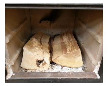
Figure 5 Logs Laid in Fire Box
